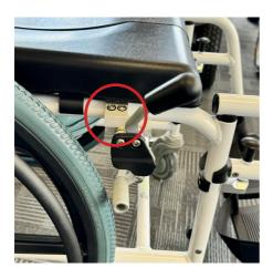
2. Adjust the brake mechanism so that the brake shoe presses the tire at least 5mm in when the parking brake is activated. Now tighten the socket screw on the mounting jig. Push the commode forwards and press the brake, checking that the brakes are tight enough to prevent the commode from moving. **REPEAT** for opposite brake.
