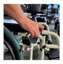
IMPORTANT! Always press the brakes on **BOTH** sides of the Shower Commode when slowing down/stopping.
