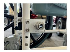
2. Push the through shaft through the 24" wheels. Press the black button in the middle of the 24" wheel to insert the wheel via the through shaft into the axle hole. Release the button again.
