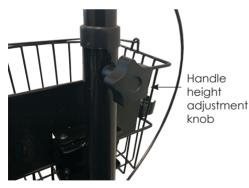
2. To adjust the handle height, loosen the handle height adjustment knob by turning it counter clockwise until it can be removed. Adjust the handle grip to the desired height and reinsert the adjustment screw into the hole, turn it clockwise until it is tightened.
